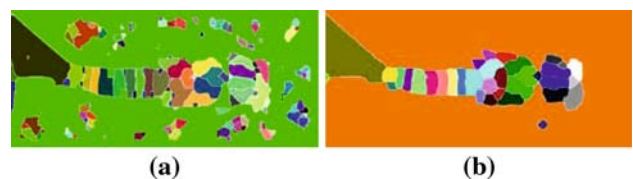
Fig. 2 a Watershed segmentation of original eigenvalue image (Fig. 1b). b Detection results using the “clean” principal curvature image (Fig. 1c)
